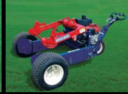
Brouwer RollMate 2430 Walk Behind Turf Installer. Excellent for Big Roll Installation.
