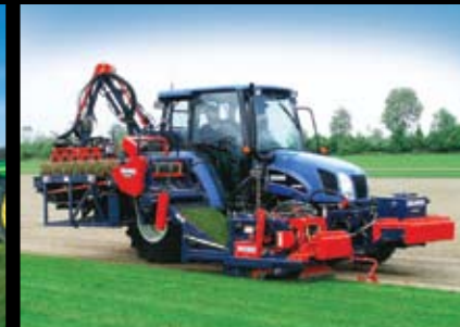
Brouwer RoboMax II. Automatic small roll harvester 16 & 24 in. Optional tracks available.
